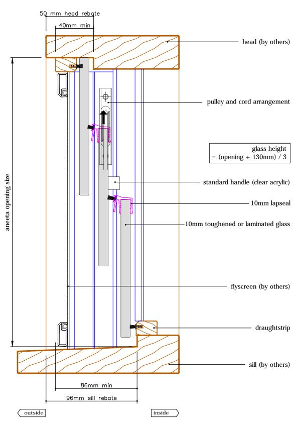
FSdF Alternative Option fixed drawing: VS 3P10 FSF T h - medium box
