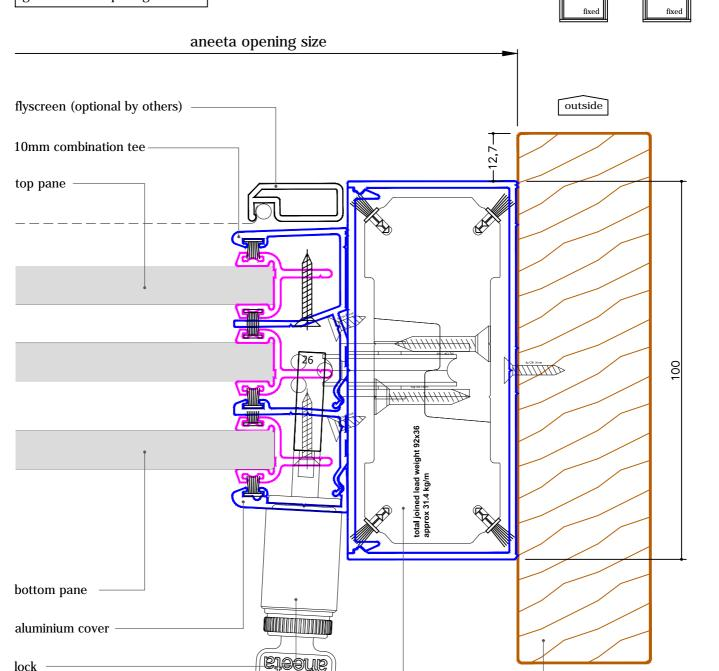
100 x 45mm box containing lead weight to counter balance moving pane of glass
